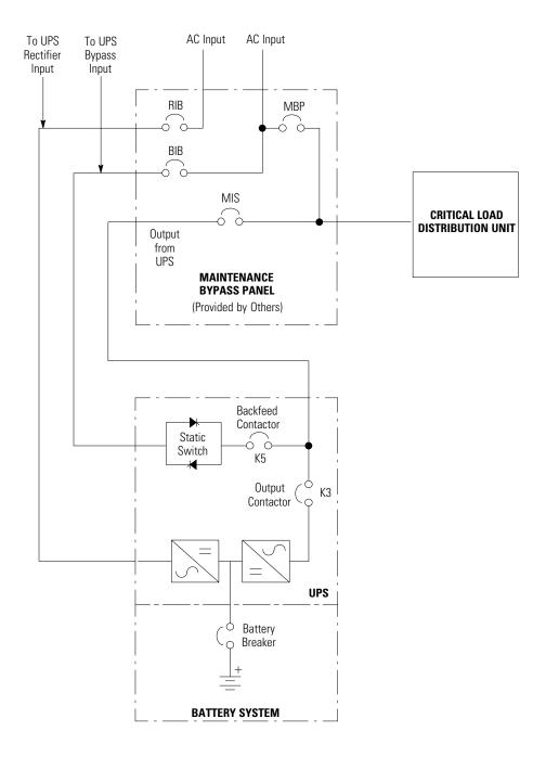
RIB: Rectifier Input Breaker BIB: Bypass Input Breaker
